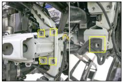
5. Install supplied washers between frame rail and the upper two crash beam mounting holes. Then reinstall the factory bolts. 將附件華司置入車體大樑及內鐵支架間的上端鎖點,完成後沿用原廠螺絲將內鐵鎖上。
