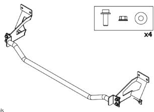
6. Install supplied brackets between frame rail and the lower two crash beam mounting holes.
