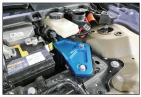
5. Reinstall the front truck and make sure the red pipeline is not pressed.
