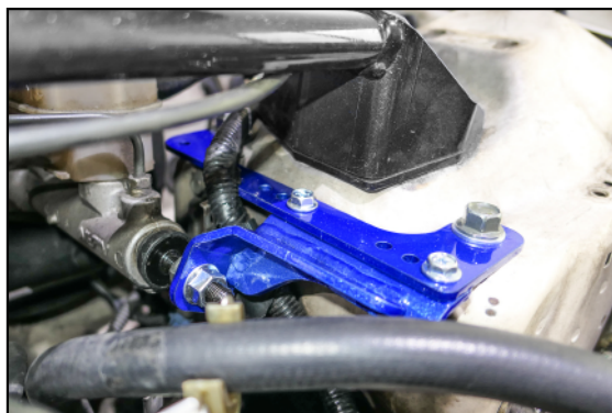
Illustration of installed state 安裝完成示意圖
