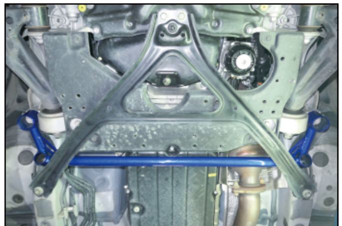
Illustration of installed state 安裝完成示意圖
