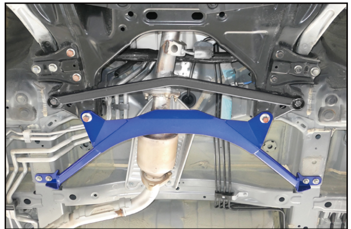
Illustration of installed state 安裝完成示意圖
