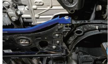
2. Install Brace by inserting its openings into the control arm bolts. Then tighten the bolts to secure the brace.
