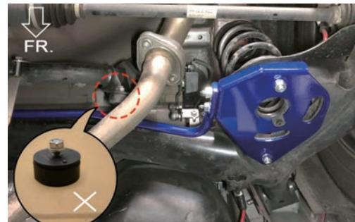
3. Install supplied ④Allen bolts & ⑦Washers (4pcs) to the spring mounts from the top on both sides. (See figure 2)
