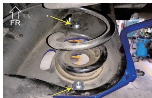
4. Tighten the bolts using supplied ⑤Nuts & ⑦Washers (4pcs) from the bottom to secure the sway bar.
