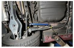
2. Install Brace to the vehicle, then reinstall the bolts to secure the brace. 安裝 結構桿,並鎖回螺絲以將桿身固定。
