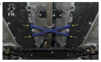
3. Once in place, reinstall the removed factory bolts to secure the brace.
