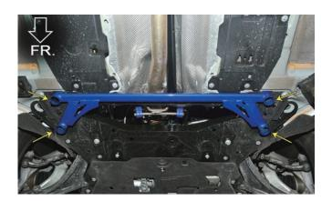
3. Once in place, install supplied ②bolts & ③washers to the front mounting holes , then reinstall the removed factory bolts to the rear to secure the brace. (See figure 2)
