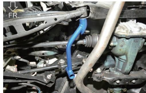
2. Insert supplied nut plates to the rear lower front (toe) control arm mounts. Align the nuts to the second holes, then Install supplied bolts and washers to secure the braces.
