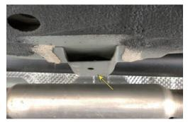
2. Position 1Brace to the vehicle, then install supplied 2Nuts, 3bolts and 4Washers to secure the brace. (See figure 2&3)
