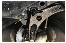
2. Install ①Brace to the vehicle, then reinstall the removed bolts to secure the brace. (See figure 2&3)
