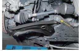
2. Place ①Brace to the vehicle and reinstall the removed bolts.to secure the brace. (See figure 2&3)
