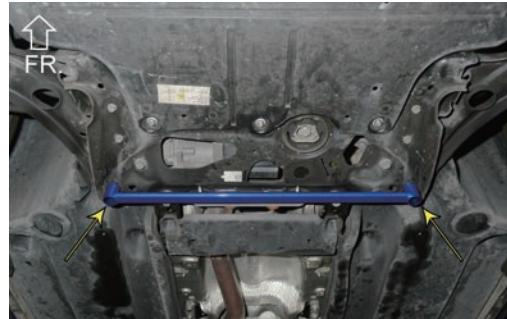
2. Install Brace to the vehicle, then reinstall the bolts to secure the brace.
