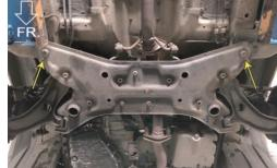
2. Install ①Brace to the vehicle using the removed bolts. (See figure 2&3)
