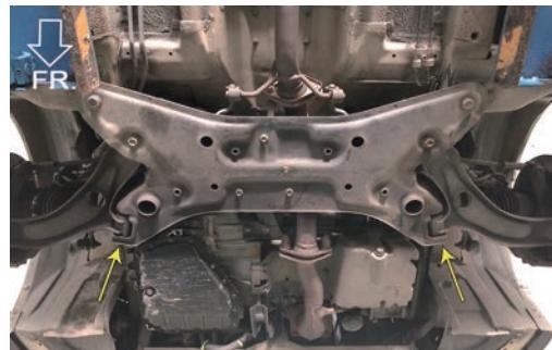
2. Position ①Brace to the sub-frame with one of the openings inserted to the loosened bolt, then install and tighten the bolts on both sides to secure the brace. (See figure 2&3)
