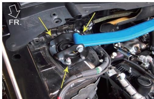
2. Place ①Strut brace on the strut towers.
