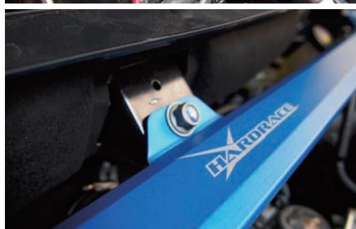
3. Once in place, reinstall the removed bolts and nuts to secure the brace.
