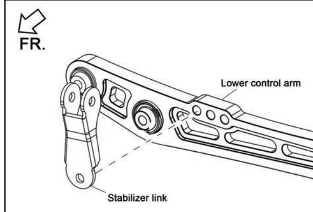
2. Reinstall the stock stabilizer links to lower control arms with the stabilizer link spacers as shown in figure 2 and tighten the supplied bolts and nuts.
