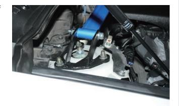
2. Position ① Strut brace over the mounts and tighten the nuts back.
