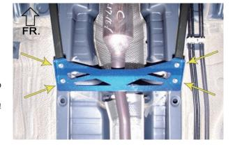
Illstration of installed state 安裝完成示意圖
