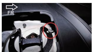
2. Remove the rear and outermost bolts of sturut mounts, then loosen the forwardmost bolts but do not remove them entirely to avoid struts from moving.
