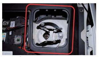
3. Position ① Strut brace over the mounts. Holes with openings on the brace should be inserted into the loosened bolts.
