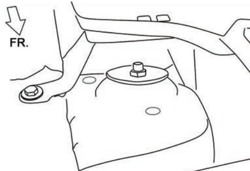
2. Position ① Strut Brace over the mounts and place ② Bolts into the holes.
