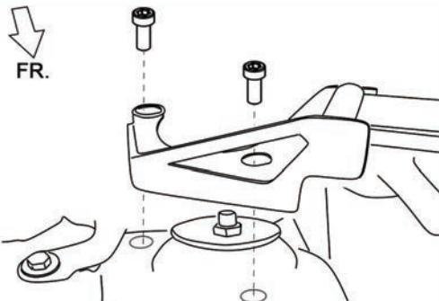
3. Tighten the bolts from inside of wheel arches using ③ Nuts (Circled), and install the wheels back.
