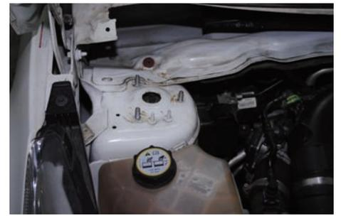
4. Position ① Strut brace over the mounts and tighten the nuts back. 將 ① 引擎室拉桿放置在避震器上座並鎖回上座螺帽。
