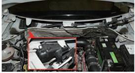
2. Position ① Strut brace over the mounts and tighten the nuts back.
