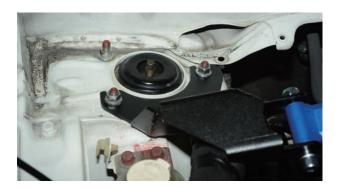
2. Remove the forward and innermost nuts of strut mounts on both sides, then place ② Washer into the studs
