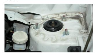
4. Tighten all the nuts, install wiper linkage, cowl panel and wiper arms (Illstration of installed state) 鎖回所有上座螺帽並裝回兩刷連桿、兩刷蓋板及兩刷臂。 (完成示意圖)
