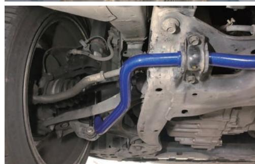
3. Position ①Stabilizer bar to the vehicle, then reinstall the removed bushing clamp bolts and end links nuts. (See figure 2)
