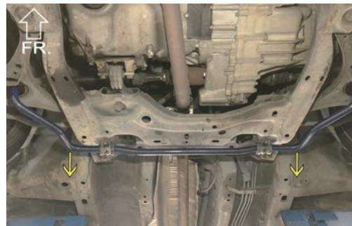
2. Assemble supplied ②Stabilizer bushings and the factory bushing clamps to ① Stabilizer bar.
