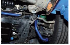
Torque of bolts. 螺絲鎖緊扭力: M8-60Nm M10-80Nm M12-100Nm M14-160Nm
