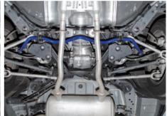
Torque of nuts for brackets: 60Nm Torque of nuts for end links: 60Nm
