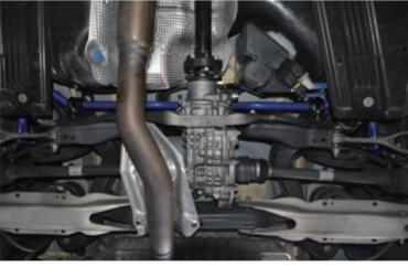
Torque for bolts 螺絲鎖緊扭力: M8-60Nm M10-80Nm M12-100Nm M14-160Nm
