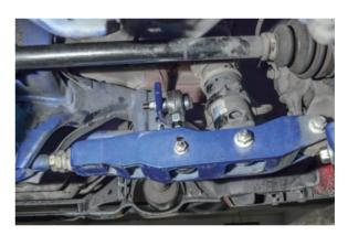
Torque of M10 bolt is 70Nm 螺絲M10鎖緊扭力為70Nm
