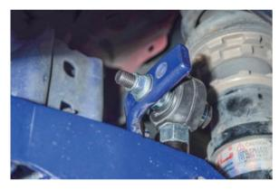
The hex bolts are used to connect the rear sway bar and stabilizer links. 配件內螺絲為李仔串連接防傾桿使用
