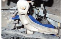
It is suggested to remove the front subframe before installation, and then remove the factory sway bar obliquely.
