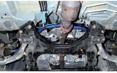
Torque for bolts 螺絲鎖緊扭力: M8-60Nm
