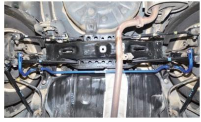
Torque for bolts 螺絲鎖緊扭力: M8-60Nm M10-80Nm M12-100Nm M14-160Nm
