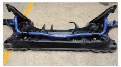
Torque for bolts 螺絲鎖緊扭力: M8-60Nm
