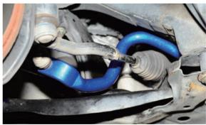
Removal of front subframe is required before installation. Please do 4 wheels alignment after installation. 需拆卸前工字樑以便完成更換防傾桿,更換完畢須完成四輪定位校正
