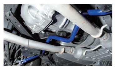
Torque for bolts 螺絲鎖緊扭力: M8-60Nm M10-80Nm M12-100Nm
