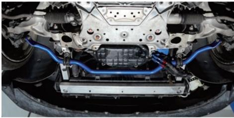
Torque for bolts 螺絲鎖緊扭力: M8-60Nm M10-80Nm M12-100Nm
