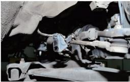
Torque for bolts 螺絲鎖緊扭力: M8-60Nm M10-80Nm M12-100Nm M14-160Nm
