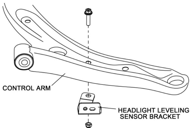
2. Install supplied bolt, nut and washer to secure the bracket.
