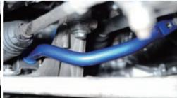
Torque for bolts 螺絲鎖緊扭力: M8-60Nm M10-80Nm M12-100Nm M14-160Nm
